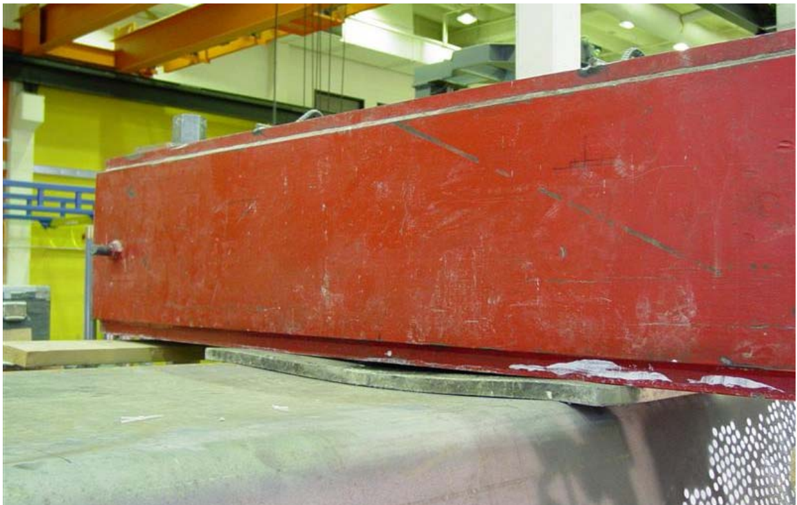
Figure 3-7 Top flange during loading
