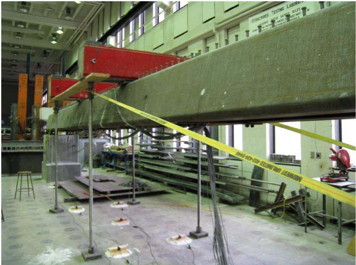
Figure 3-35 Folded plate girder test B1 setup
