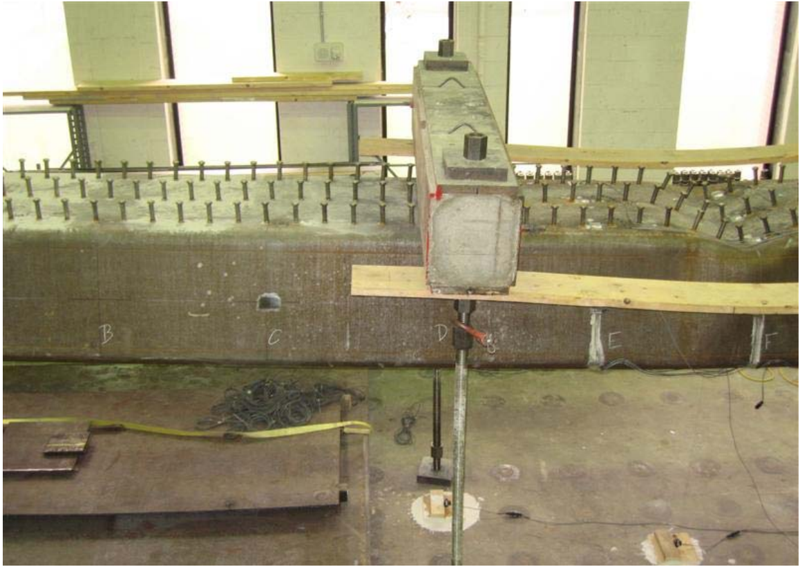
Figure 3-47 Permanent deformation after unloading
