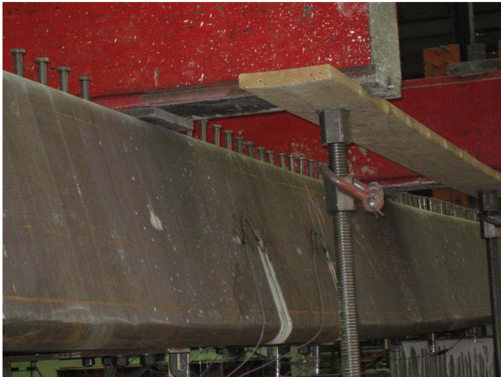
Figure 3-40 Test B1 web at 140kip
