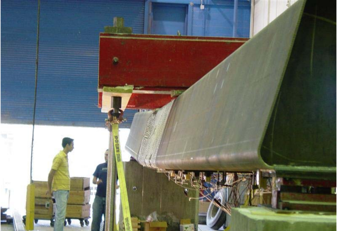
Figure 3-11 North side of girder facing east showing girder deflection and web buckling
