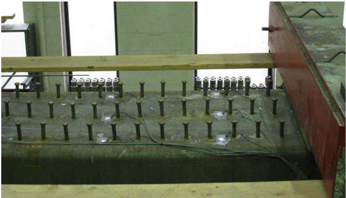
Figure 3-37 Top flange at twice the construction moment
